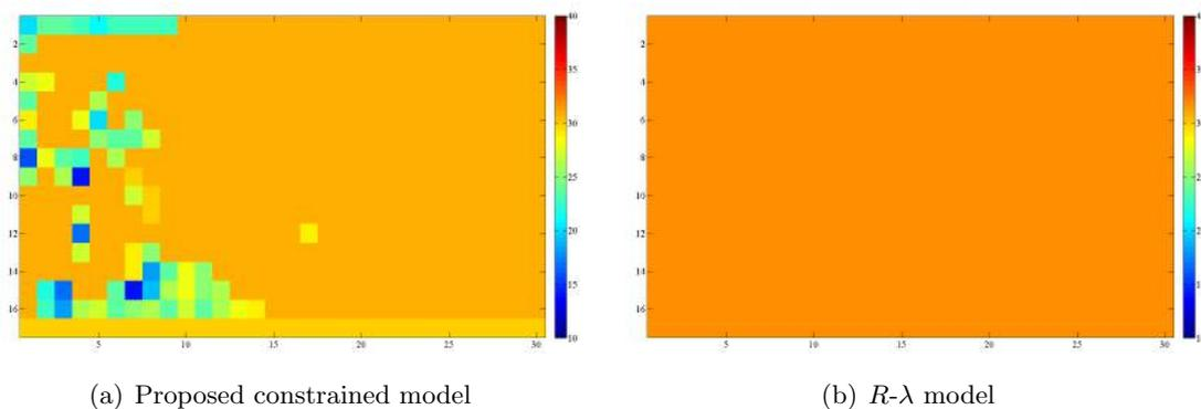
Figure 5.18: Comparison of obtained QP maps using proposed constrained model and  $R-\lambda$  model of an inter-coded frame of “BasketballDrive” sequence
