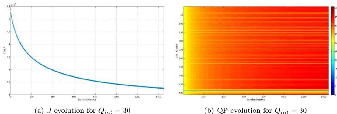
Figure 5.13: Evolution of frame cost  $J$  and QP of all CTUs over gradient descent algorithm iterations at high bit rate
