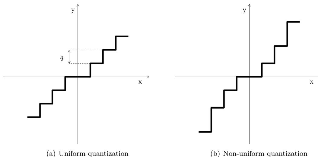
Figure 1.3: Input-output characteristic of uniform and non-uniform quantizer
