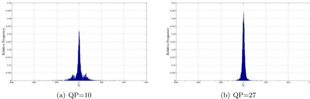
Figure 5.6: Impact of QP on transform coefficients’ histograms of and intra coded CTUs
