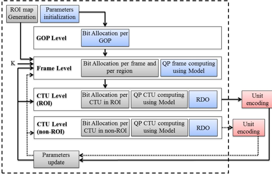
Figure 7.1: ROI-based rate control scheme for HEVC
