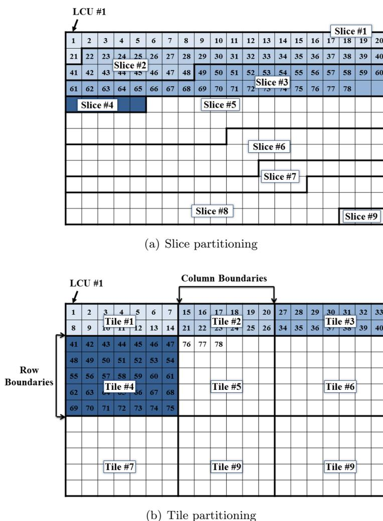
Figure 2.4: Examples of slice-based and tile-based partitioning
