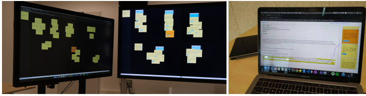
Fig. 7. Two different affinity diagrams on two large displays, and a coding view opened in a laptop. Long press a note in any of them highlights notes with same content in the others.
