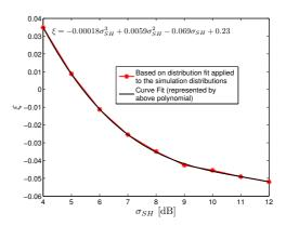
Fig. 6. Shape parameter  $\xi$  of GEV distribution versus  $\sigma_{SH}$  for R=1500 m,  $P_{Tx}=43$  dBm and reuse 3x3x3.
