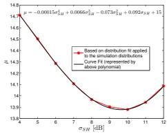
Fig. 8. Location parameter  $\mu$  of GEV distribution versus  $\sigma_{SH}$  for R=1500 m,  $P_{Tx}=43$  dBm and reuse 3x3x3.
