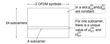
Fig. 3. Shadowing and fast fading over a PUSC slot.
