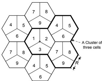
Fig. 2. Frequency Reuse Pattern 3x3x3 ( $R$  is the cell range).
