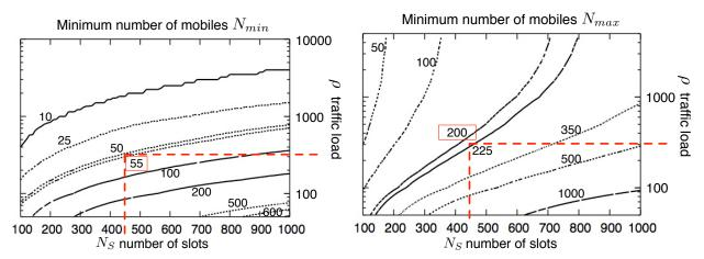
(a) Dimensioning the minimum value of N for having  $\bar{U} \geq$  (b) Dimensioning the maximum value of N for having  $\bar{X} \geq$  50%.
