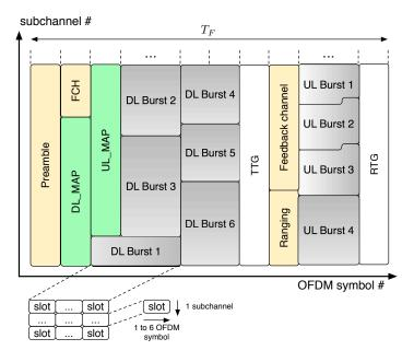
Figure 1.1: TDD frame structure.
