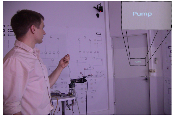
Figure 2: The Robotic Arm (RA) technique. The robotic arm is initially oriented towards the door and displays the name of the target.
