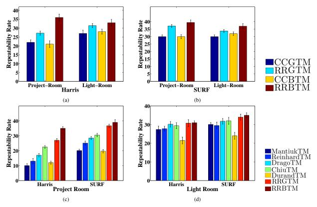
Figure 4: Row 1. (a) and (b) Average repeatability score and standard deviation for both correlation and response based optimized approaches using Harris and SURF detector respectively. Row 2. (c) and (d) Average repeatability score and standard deviation for the reflectance models (GTM and BTM) and other commonly used TMs on Project Room and Light Room dataset
