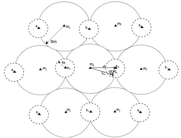
Fig. 3. Instance of scenario deployment for  $d = R_m$ .
