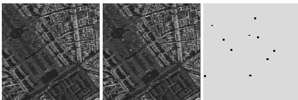
(b) Realistic SAR synthetic images. From left to right: synthetic image y_t , Synthetic image y_{t'} and the reference map of changes.
