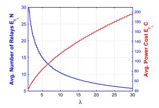
**Fig. 6.** Average number of relays  $\mathbb{E}_{\pi_{\lambda}^{i}}N$  (left scale; curve labeled (2)) and average power cost  $\mathbb{E}_{\pi_{\lambda}^{i}}C$  (right scale; curve labeled (1)) as a function of  $\lambda$  (p = 0.002, q = 0.5 and  $\eta = 2$ ).
