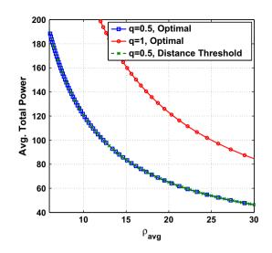
**Fig. 11.** Average total power as a function of  $\rho$  for the optimal policy  $(q = 0.5 \text{ and } q = 1, \text{ which corresponds to the straight line) and for the heuristic <math>(q = 0.5)$  for p = 0.002 and  $\eta = 2$ .
