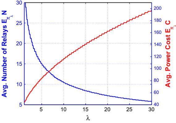
**Fig. 6.** Average number of relays  $\mathbb{E}_{\pi_\lambda} N$  (left scale; curve labeled (2)) and average power cost  $\mathbb{E}_{\pi_\lambda} C$  (right scale; curve labeled (1)) as a function of  $\lambda$  ( $p = 0.002$ ,  $q = 0.5$  and  $\eta = 2$ ).
