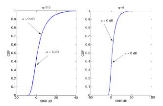
Fig. 4. CDF of the SINR with  $\eta=3.5$  (left) and  $\eta=4$  (right), for a Poisson model network and standard deviations of the shadowing values comprised between 0 dB (no shadowing) (curve in the left of each figure) and 8 dB (curve in the right of each figure). For readability, only the values of 0 and 8 dB are indicated in the figure. The curves between these two curves represent the cases 3 dB, 6 dB. They are in the line thickness
