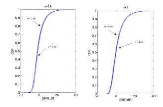
Fig. 3. CDF of the SINR with  $\eta=2.6$  (left) and  $\eta=3$  (right), for a Poisson model network and standard deviations of the shadowing values comprised between 0 dB (no shadowing) (curve in the left of each figure) and 8 dB (curve in the right of each figure). For readability, only the curves drawn with  $\sigma=0$  and 8 dB are indicated in the figure. The curves between these two curves represent the cases  $\sigma=3$  dB, 6 dB. They are in the line thickness
