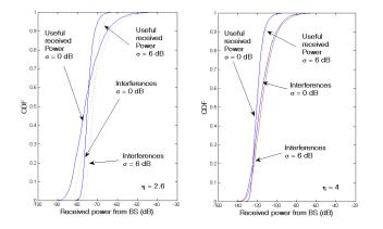
Fig. 5. CDF of the useful signal and the interferences, for  $\eta = 2.6$  (left) and  $\eta = 4$  (right), without shadowing ( $\sigma = 0$  dB, blue continuous curves) and with shadowing ( $\sigma = 6$  dB, red dotted curves)
