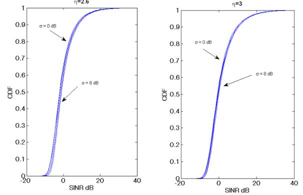
Fig. 3. CDF of the SINR with  $\eta = 2.6$  (left) and  $\eta = 3$  (right), for a Poisson model network and standard deviations of the shadowing values comprised between 0 dB (no shadowing) (curve in the left of each figure) and 8 dB (curve in the right of each figure). For readability, only the curves drawn with  $\sigma = 0$  and 8 dB are indicated in the figure. The curves between these two curves represent the cases  $\sigma = 3$  dB, 6 dB. They are in the line thickness
