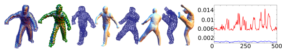
Figure 17: Encoding with a reference cage generated automatically . The surface is first voxelized. We then contour a slight offset of this volume before simplifying it using QSlim .
