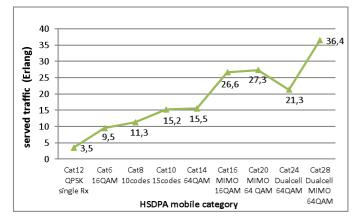
Figure 6. Streaming capacity for all HSDPA device categories (on 10 MHZ)
