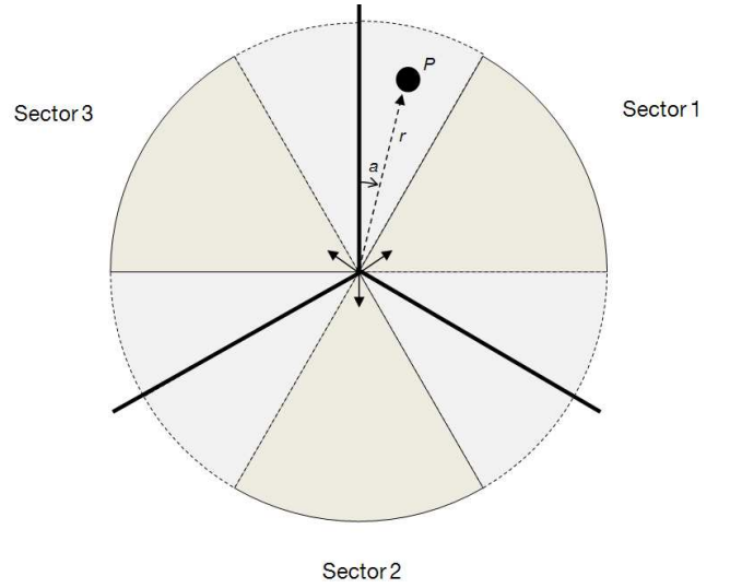
Fig. 1. A tri-sectored site.
