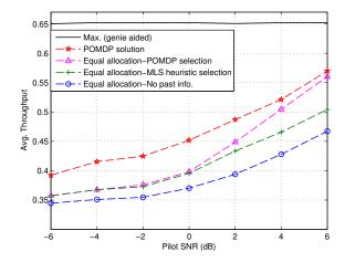
Fig. 6. Avg. Throughput vs. Pilot SNR for FSMC model ( $N=4,\,L=4,\,G=4,\,{\rm data}$  SNR = 0 dB,  $f_dT_f=0.01$ ).
