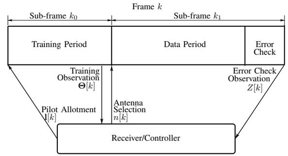
Fig. 3. Sequence of operations in frame  $k$ .
