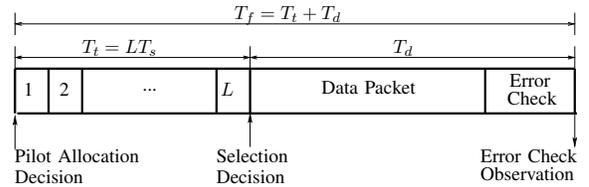
Fig. 1. Frame structure for training and data reception.
