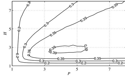
Fig. 5. Contour of the asymptotic performance of regular (3,6)-LDPC codes in AIN channel for  $\alpha = 1.2$ .
