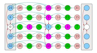
**Fig. 1.** Example of MVC prediction structure with intra- (horizontal arrows) and inter-view (vertical arrows) prediction. The numbers indicate the coding order.
