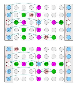
**Fig. 3.** Two possible schedules (first 20 rounds). The numbers indicate the round in which the frame is included in the coding window. The dashed border identifies which frames have not been selected yet for inclusion in the coding window at the 20-th round.
