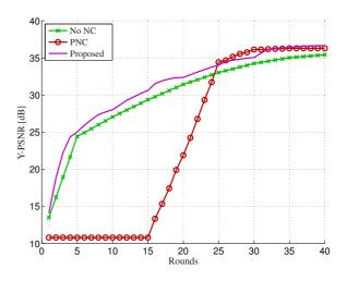
**Fig. 5**. Comparison of the average Y-PSNR of the decoded sequences, for 2 sources and packet loss probability 10%.
