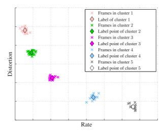
**Fig. 2.** Clustering of video frames for RDO-scheduling. Frames with similar operating points are assigned to the same cluster. The RDO-scheduling will consider each frame as having the average operating point of its cluster.
