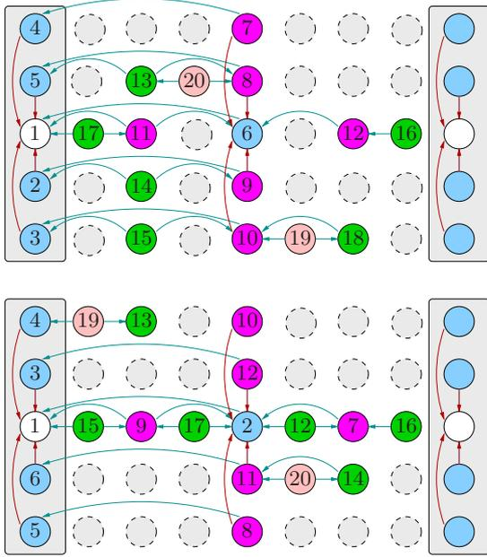
**Fig. 3.** Two possible schedules (first 20 rounds). The numbers indicate the round in which the frame is included in the coding window. The dashed border identifies which frames have not been selected yet for inclusion in the coding window at the 20-th round.
