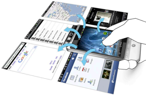
Figure 9. An example of an implementation of JerkTilts for switching among applications.
