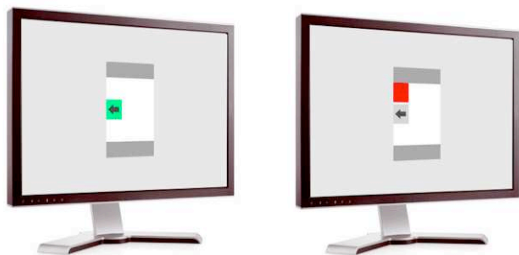
Figure 5. Examples of the feedback delivered on an external screen after a selection classified by the system as correct (left) and incorrect (right). The gray arrow indicate the intended tilt direction.
