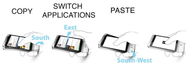
Figure 10. An example of a copy-and-paste operation between two different applications. A JerkTilt to the South copies whatever object is under the thumb; a JerkTilt to the East switches applications; a JerkTilt to the South-West pastes the object at the location designated by thumb contact.
