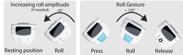
Figure 2: Example of a roll gesture. Left: a preparatory back-roll for increasing the total roll movement. Right: Execution of the roll gesture (the trigger being kept pressed).
