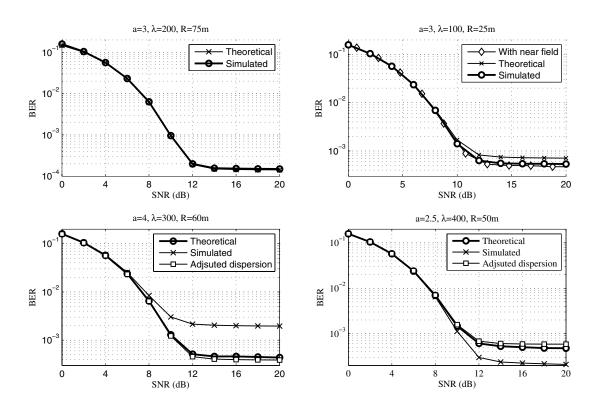
Fig. 3. Comparison between semi-analytical and simulated BER in different situations with a rectangular pulse. The signal to noise ratio is the ratio between the useful signal power and the thermal noise power at the receiver, not including the multiple access noise.
