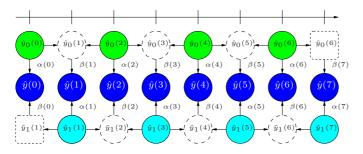
Figure 1. Structure of central decoder. Solid circles represent received frames; dashed circles represent interpolated frames. Horizontal arrows represent interpolation. Vertical arrows represent weighted sum. With  $\hat{y}_n(k)$  we denote the *k*-th frame of description *n*. For each k,  $\beta(k) = 1 - \alpha(k)$ .
