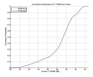
Figure 6. Cumulative distribution function of the Y-PSNR of the decoded frames (Bitrate  $1.0\,\rm Mbps, \sim 25\,\%$  of packets lost).
