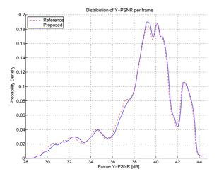
Figure 5. Probability density function of the Y-PSNR of the decoded frames(Bitrate  $1.0\,\rm Mbps,\sim25\,\%$  of packets lost).
