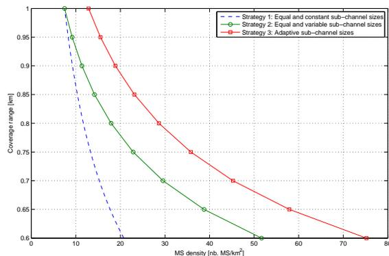
Figure 9: Effect of MS density increase on the cell coverage with a fixed number of sub-carriers per subchannel (solid) or with variable number of sub-carriers (circles) ( $\tilde{D} = 256$  kbps,  $P_{out} = 2\%$ ,  $W_{sc} = 11$  kHz,  $\sigma = 6$  dB,  $R_c = 1$  km).
