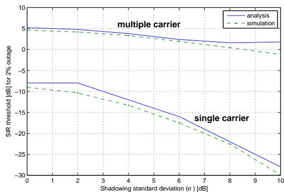
Figure 7: SIR threshold  $\delta$  in the cell ( $r = R_c/2$ ) for 2% outage probability as a function of the shadowing standard deviation; comparison between analysis (solid curves) and simulations (dotted curves) on a hexagonal network ( $N_{sc} = 48$ ,  $\eta = 3$ ).
