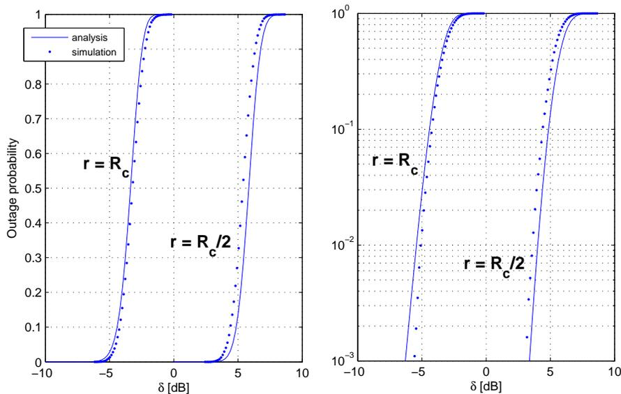
Figure 5: Outage probability at cell edge ( $r = R_c$ ) and inside the cell ( $r = R_c/2$ ); comparison between analysis (solid curves) and simulations (dotted curves) on a hexagonal network ( $N_{sc} = 48$ ,  $\eta = 3$ ,  $\sigma = 3$  dB).
