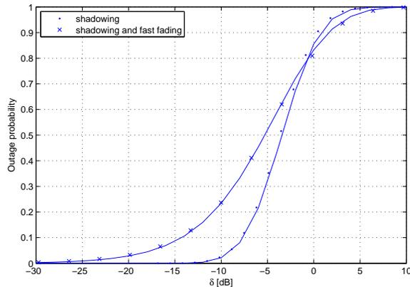
Figure 4: Impact of fast fading on the outage probability for a mobile located at cell edge ( $r = R_c$ ,  $\eta = 3$ ,  $\sigma = 3$  dB), dotted curves are obtained with simulations solid ones with analysis.
