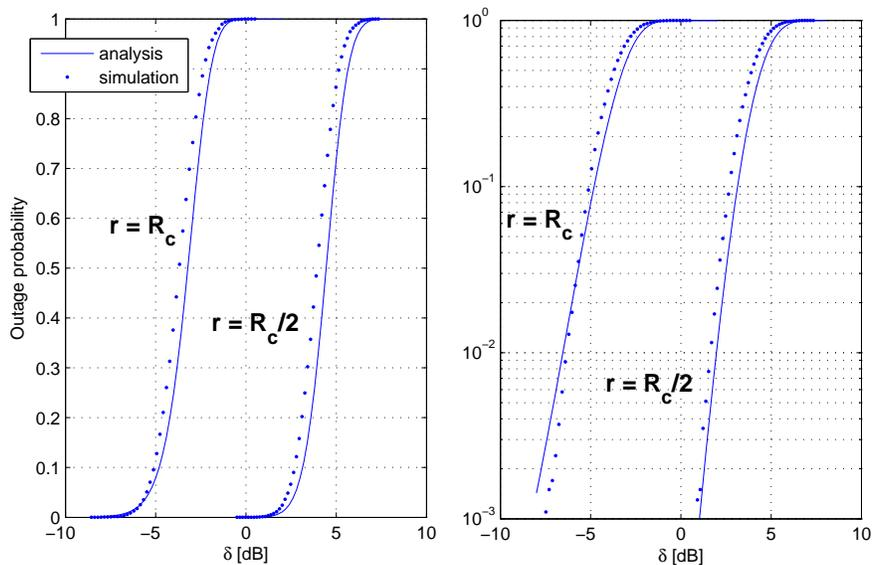
Figure 6: Outage probability at cell edge ( $r = R_c$ ) and inside the cell ( $r = R_c/2$ ); comparison between analysis (solid curves) and simulations (dotted curves) on a hexagonal network ( $N_{sc} = 48$ ,  $\eta = 3$ ,  $\sigma = 6$  dB).
