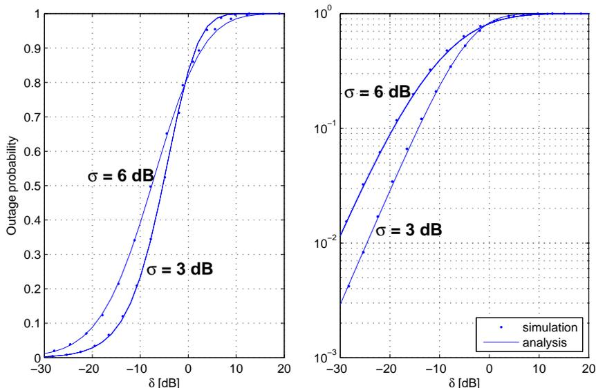
Figure 3: Outage probability for a mobile located at cell edge ( $r = R_c$ ); comparison between analysis (solid curves) and simulations (dotted curves) on a hexagonal network ( $\eta = 3$ ); zoom on the right.
