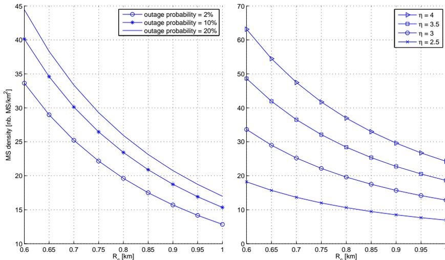
Figure 11: Influence of the outage probability (left) and the path-loss exponent (right) on the cell capacity as a function of the half-distance between BS ( $\tilde{D} = 256$  kbps,  $W_{sc} = 11$  kHz,  $\sigma = 6$  dB, strategy 3)  $\eta = 3$  (left),  $P_{out} = 2\%$  (right).
