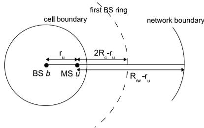
Figure 13: Integration limits for external interference computation.
