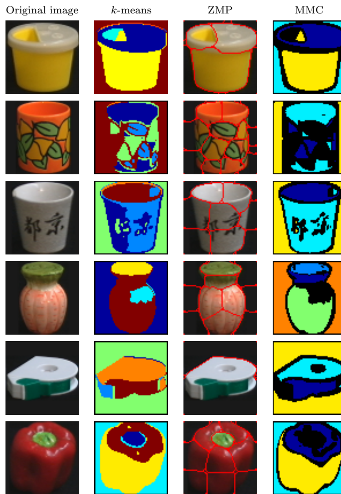
Figure 12: Comparison of image segmentations from 3 \times 3 color patches. Results with k -means were obtained by tuning k by hand. In all examples, for maximal meaningful clusters non-detected areas are depicted in black.
